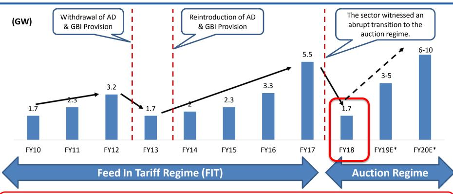
Impact of the abrupt transition to auction Regime from FIT regime seen in wind installations in FY18. The impact of 9.7 GW auctions conducted over the last 16 months would be visible in installations in FY19-20.
